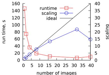
Figure 1: Calculating  $\pi$  on 2 nodes - scaling.
