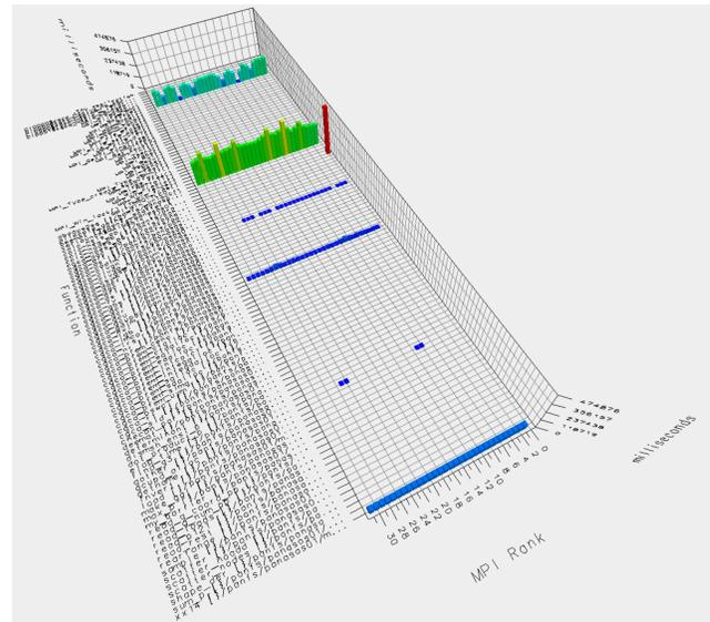
Figure 12: 3D profiling bar chart of program xx14std, coarray+MPI, on 2 nodes with 32 images.
