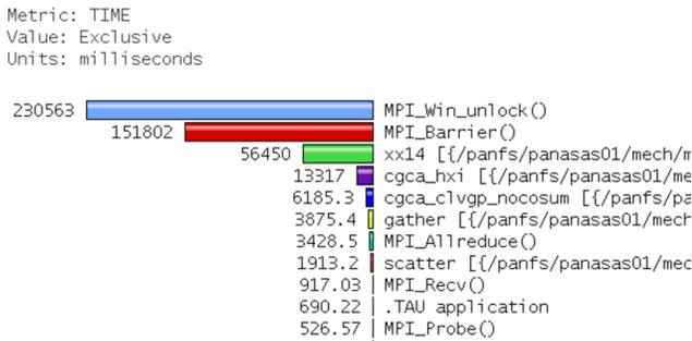
Figure 14: Profile of program `xx14std`, `coarray+MPI`, on a single image.
