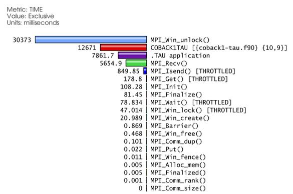
Figure 7: Profile of coback1-tau on a single image.
