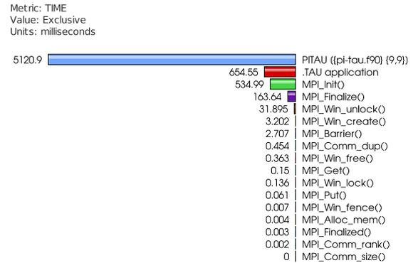
Figure 3: Calculating  $\pi$  - single image profile.
