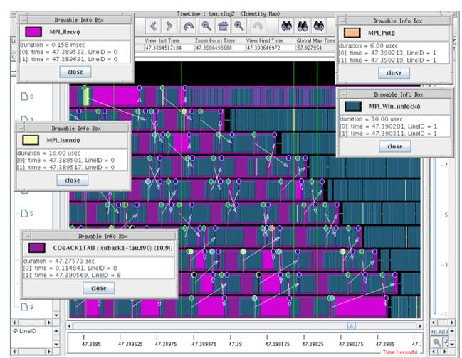
Figure 8: A fragment of the trace of the Laplacian code coback1-tau on 10 images.
